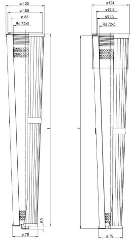
with self-adhesive polyester felt with cavity free silicone mould seal seal
