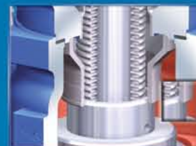
3. Rugged plug / stem guide – permits higher differential pressures
