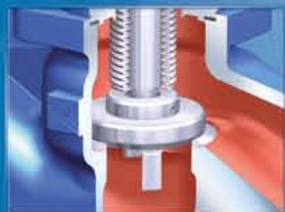
3. Additional stem guide via the V-port plug (permits higher differential pressures)
