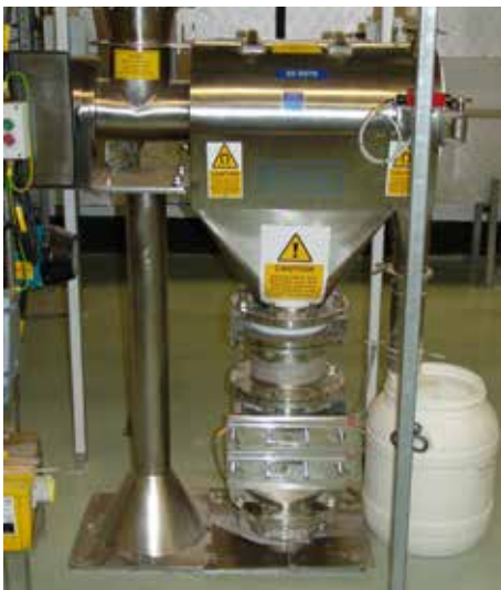
Pharmaceutical specification double row housed easy clean grid, pre and post sifter protection.
