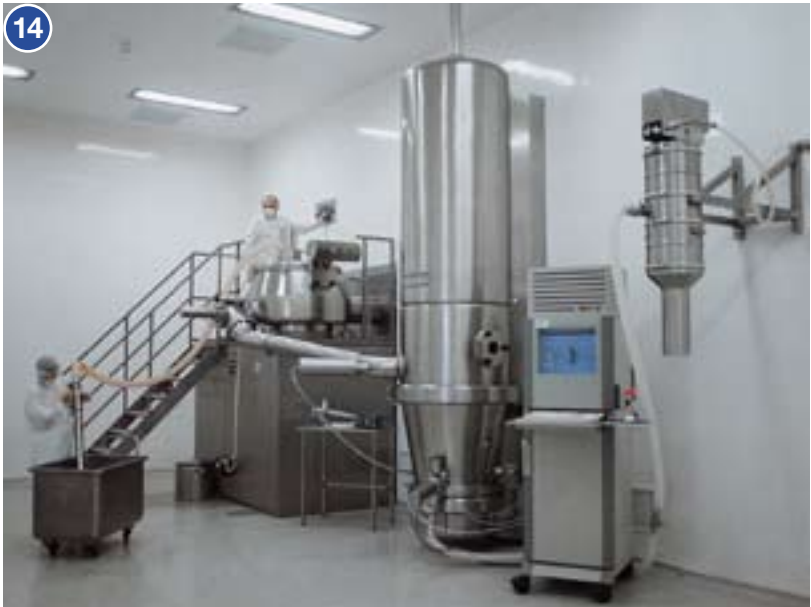
Fig. 14: Vacuum Conveyor for the automatic discharging of a fluidized bed dryer. Product delivery through a submersion tube into IBCs.
