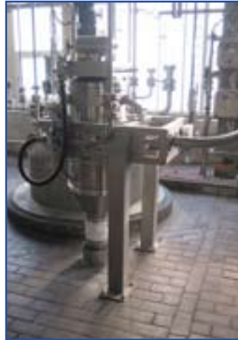
Volkman Conweigh System to convey and dose powders into a chemical process vessel
