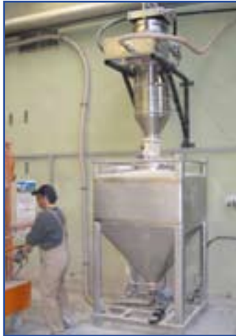
Volkman Conweigh System for feeding the components of a recipe into an IBC; ceramic industry application
