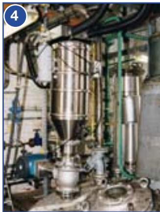
Fig. 1: Vacuum Conveyor in Pharma design, with inertizing done at the suction lance and complete inerting sequence done by a pneumatic control. Multijector Vacuum pump inside the controller box.
