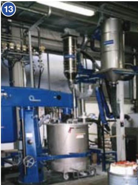
Fig. 8: Filling of toner powder into cartridges with a Vacuum Conveyor VR315.
