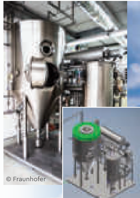
SPRAY DRYER EXPERO SDL-06 in pilot plant for chemical products
