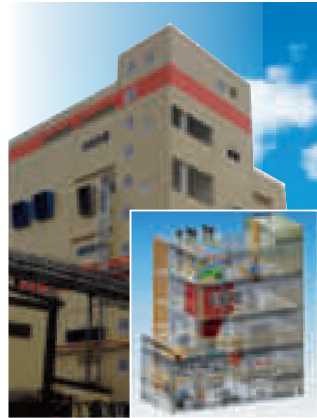
SPRAY DRYER MULUS 3SSD in the starch industry for maltodextrin with external fluid bed
